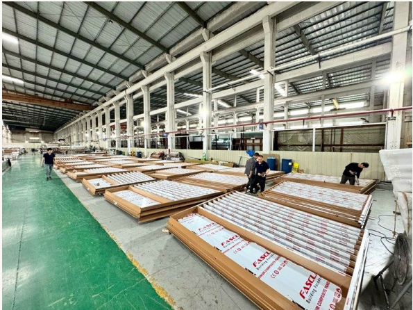
FIG. 03 · PRE-FABRICATED FAÇADE UNITS STAGED FOR SHIPMENT FROM A CONTROLLED PRODUCTION FACILITY.
